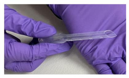
Close the end of the 10 mL syringe with a cap stopper to prevent sample from flowing out of the barrel.
