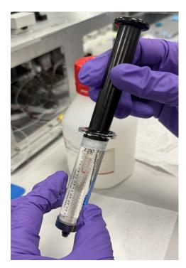
If bubbles are present, invert the syringe and leave it so that the bubbles can rise to the top.
