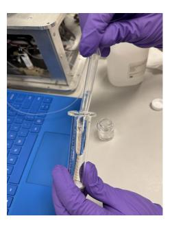
Repeat this process until there is sample at the very top of the syringe barrel. The sample should be flush with the opening.
