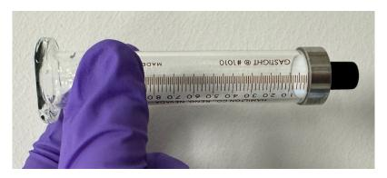
Fill the dropper with sample. Try not to have bubbles present in your sample. Note: depending on the sample this may be difficult to accomplish. Proceed with loading the sample anyways.
