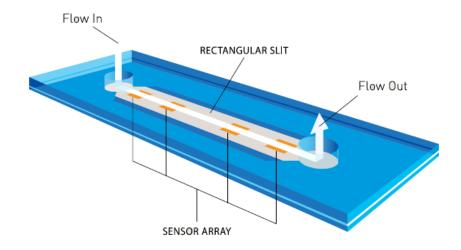
This direct and precise control of flow rate translates directly into precise control of the shear rate experienced by the sample. This is essential for accurate viscosity determination for all fluid types:
