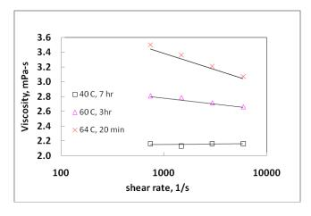
A notable change with the extent of denaturation or aggregation is that the viscosity becomes dependent on the shear rate – shear thinning non-Newtonian.
