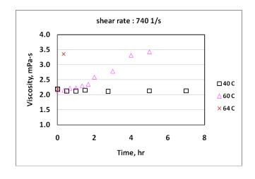
Viscosities of  $\gamma$ -globulin solutions were measured as a function of incubation time. Viscosity remained the same even after seven hours of incubation at 40  $^{\circ}\text{C}.$  However, when the solution was incubated at 60  $^{\circ}\text{C},$  viscosity started to increase within 40 mintutes. This viscosity increase suggests that proteins unfolded and even aggregated.
